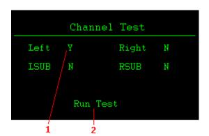
To highlight an option use the "UP" and "DOWN" navigational buttons and then press "ENTER" button to make your selection. After all selections are made, highlight the "Run Test" option and hold down the "ENTER" button to produce the test signal. The test tone will stop when the "ENTER" button is released. Press the "MENU" button to exit this menu.
