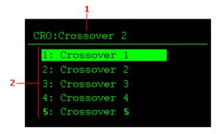
When an option is selected the system will load the crossover filter and resume to normal operation. Crossover filters are user programmable from the Crossover screen in the Room Correction Software.
