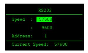
To change the system baud rate use the "**UP**" and "**DOWN**" navigational buttons to highlight the desired baud rate and then press the "**ENTER**" button to select it. The new baud rate will be displayed on the bottom of the screen.
