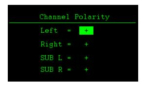
To select an option use the "**UP**" and "**DOWN**" navigational buttons and to change its value press the "**ENTER**" button to toggle between a "+" or "-" setting.
