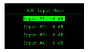
To select an option use the "**UP**" and "**DOWN**" navigation buttons and to change its value press the "**ENTER**" button to toggle between the -6dB and 0 dB selections.
