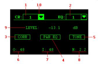
To move the cursor indicator (10) use the front panel or remote control navigation buttons. To select an option press the "**ENTER**" button.
