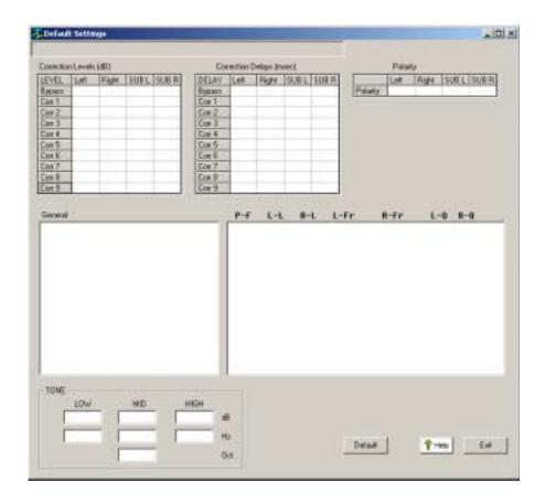
**2 -** Select the "**Default**" button and the default parameters for the RCS 2.2 X will be loaded into the RCS 2.2X. The RCS 2.2X will turn OFF and then ON and return to normal operation when finnished.
