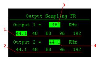
To set the sampling frequency for digital output 1, use the "**LEFT**" or "**RIGHT**" navigational buttons to highlight the desired option (on line 1) and then press the "**ENTER**" button to make the selection. The new sampling frequency will be displayed in block (3).
